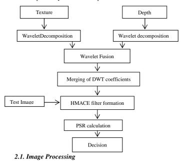
While carrying multiresolution wavelet fusion, both images have respective features
